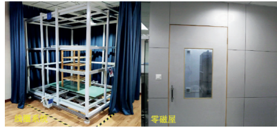
模拟地磁场变化装置(线圈和零磁屋) Magnetic coils and magnetically shielded room
