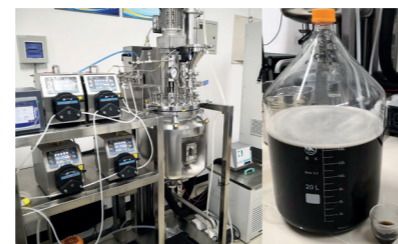
仿生合成磁性铁蛋白纳米颗粒实验平台 The experimental platform of biomimetically synthesized magnetoferritin nanoparticles
